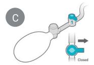
A. Check that lever (1) is turned parallel with the tube (open).
