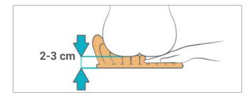
•Inflate the cushion by turning the silver valve tip counterclockwise and using the black hand pump to inflate.
