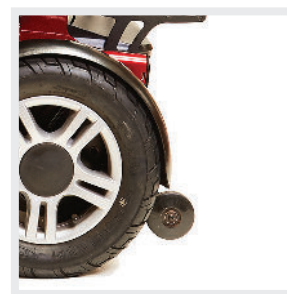
Anti-tilt wheels for stability and safety
