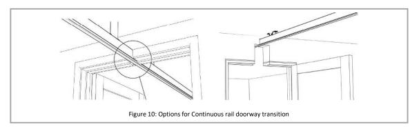
• Motor Transition: A portable motor can be moved between one track system and a second. Alternatively, a sling and suspension can be moved between one fixed motor and another
