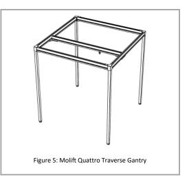
• Additional components: Tracks can be added to utilising a transition, this attachment allows for a traverse rail to transition into a straight or another traverse system eg. Moving from a traverse system in a bedroom to a straight rail in a bathroom. Switches also allow for directional changes eg. Movement from a bedroom then selecting direction towards bathroom or direction towards another room.
