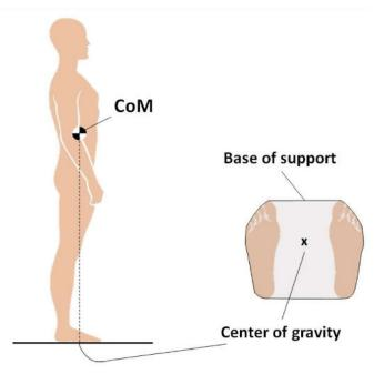
gravity must move a greater distance to fall outside the BOS). A lower COG increases stability (it's unlikely that the line of gravity will fall outside the BOS)
