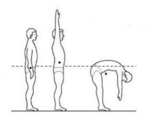
The centre of mass (COM) is the balance point of an object's mass. If a pivot were placed at this point, the object would remain in place and be balanced. The COM of a system is not always at the geometric centre of the system.
