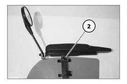
Turn the rear-view mirror on the attachment rod and ball joint until you reach the desired angle.
