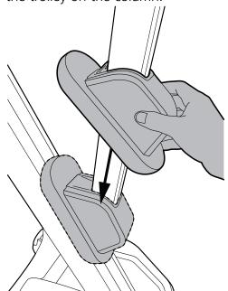
Fit the cover onto the trolley
