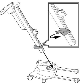
Place the cover on to the lifting column. Twist the cover sideways to make it stay on column. Insert the lifting column into the chassis.
