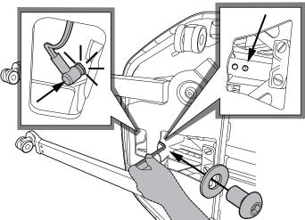
Turn the lifter over on the side. Insert screw and washer in the top hole and tighten the screw. Connect cable between column and chassis. (NB! The cable is NOT applicable with the Molift Quick Raiser 205 FL version)
