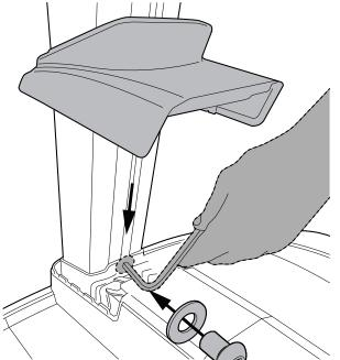
Mount the screw with washer on column. Slide the screw down to chassis, and tighten the screw.
