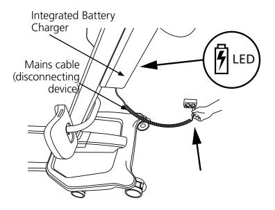
The lifter has an integrated charger. Park the lifter and connect to a wall socket to charge the battery. A LED-light on the back of the battery box will be red while charging. The LED-light on the battery box will show a steady green color when lifter is fully charged. While charging the LED-lights on the control panel will flash every 10 seconds.
