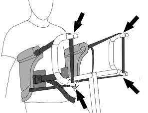
Fasten the sling to the lifting arm by guiding the strap into all 4 hooks.
