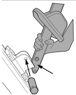
Place the cover onto the lifting arm. Place lifting arm in trolley, and insert the bolt.
