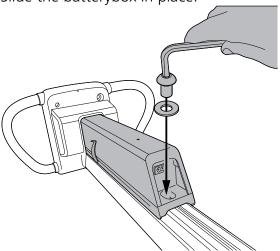
Use the allen key and tighten screw clockwise. NB! make sure to use the washer.
