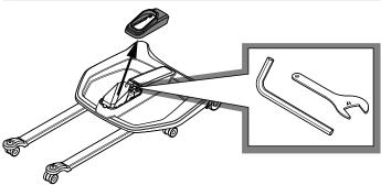
Locate assembly tools (5mm allen key, and 17mm spanner)
