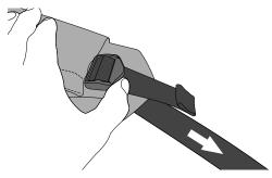
Loosen the straps again by angling the buckle and puling the strap out.
