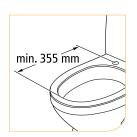
Min. 355 mm Hi-Loo fits most types of toilets. The distance from the attachment holes to the inner front edge must be minimum 355 mm.
