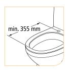
Min. 355 mm Hi-Loo fits most types of toilets. The distance from the attachment holes to the inner front edge must be minimum 355 mm.
